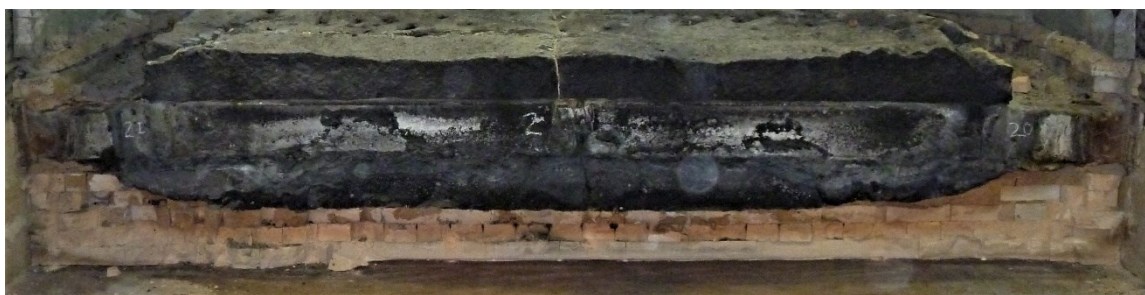
Figure 3. Cell lining cross section of Lining B design.
