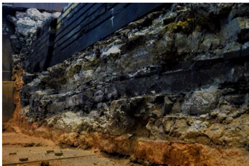
Figure 5. CBA cell lining cross section – Cell 1639 autopsy.
