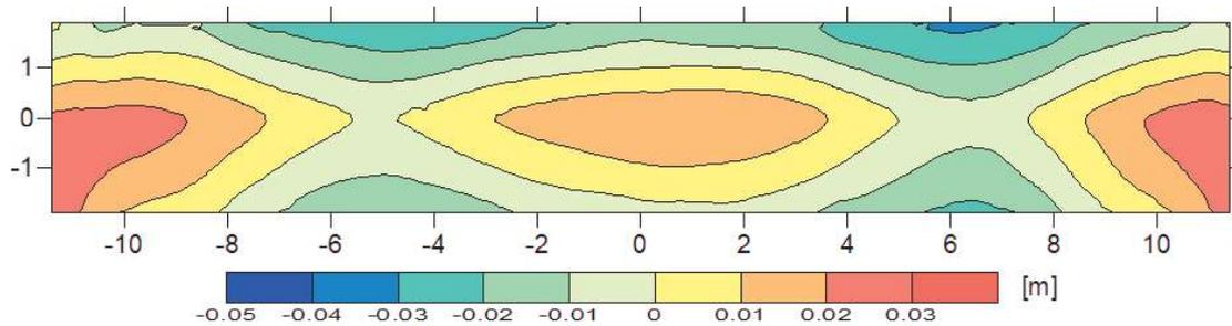
Figure 9. Metal/bath interface deformation (m). Novel cathode assembly model.
