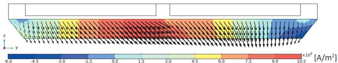
Figure 12. Metal current density vectors at the cell vertical cut. Inserted steel bar model.
