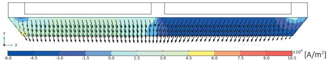
Figure 13. Metal current density vectors at the cell vertical cut. Novel cathode assembly model.
