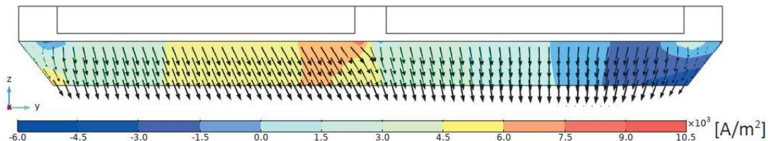
Figure 11. Metal current density vectors at the cell vertical cut. Integral copper bar model.
