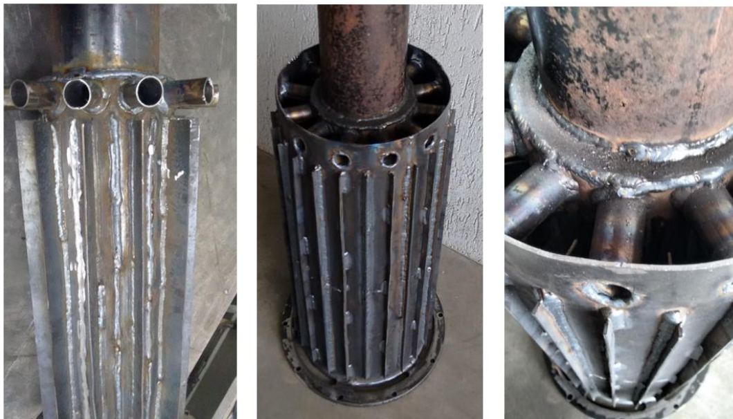
Figure 4. Prototype construction process. All fins are welded in both gas ducts and alumina duct.
