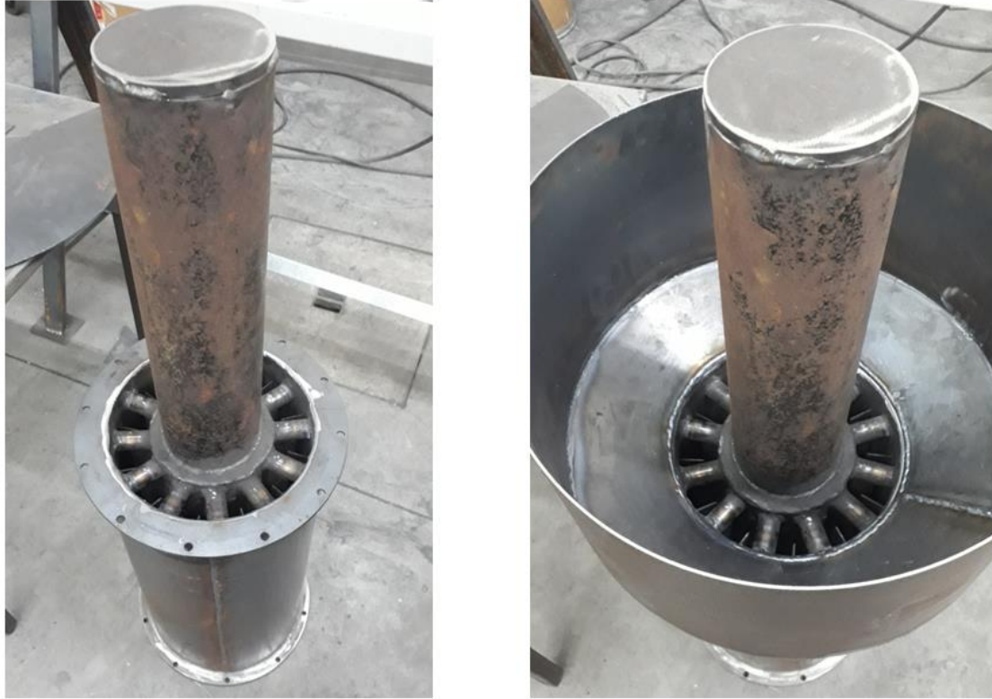
Figure 5. Left: prototype top view. Right: prototype with the alumina feeding reservoir.
