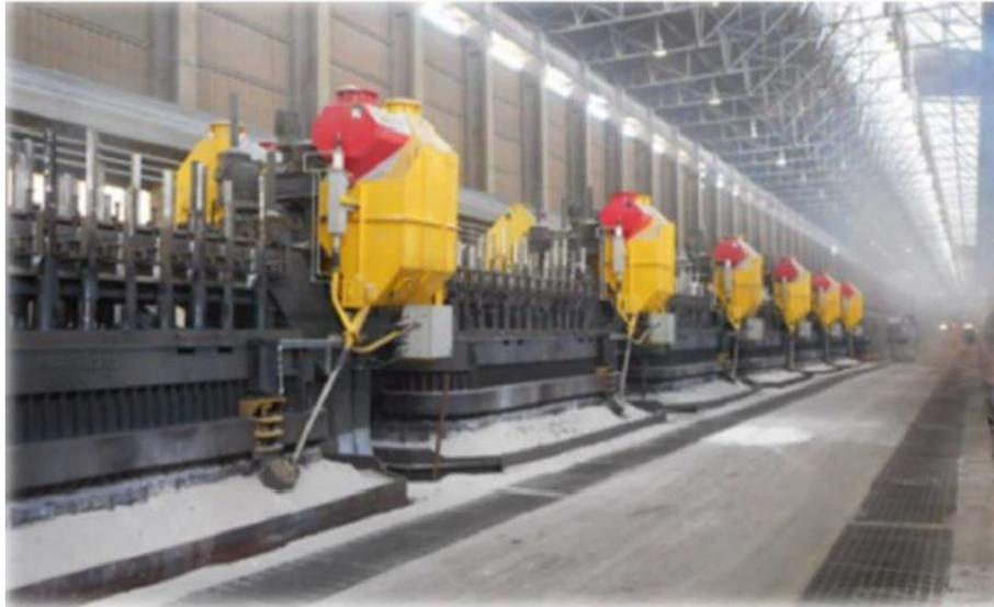
**Figure 10. Point feeder at CBA Søderberg cells, alumina duct, and feeding chute [5].**
